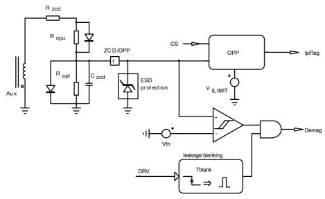
Figure 9. ZCD and OPP Circuit
