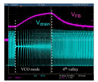
Figure 6. The Controller Hesitates Between VCO Mode and 4<sup>th</sup> Valley: C<sub>t</sub> is Too Big!
