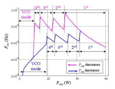
Figure 4. Switching Frequency versus Output Power at V<sub>in</sub> = 90 Vrms
