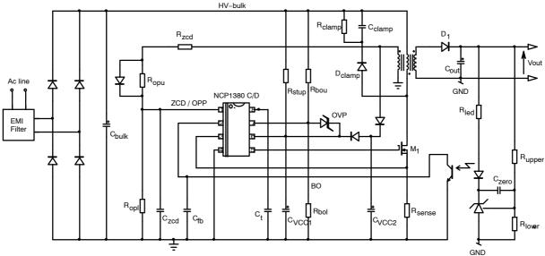
Figure 2. Application Schematic for Versions C and D
