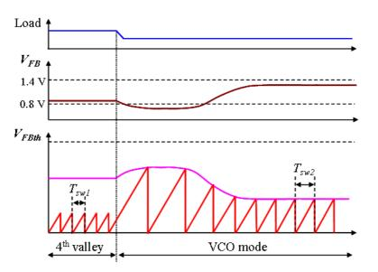
Figure 7. 4<sup>th</sup> Valley to VCO Mode Transition with an Optimum Timing Capacitor C<sub>t</sub>
