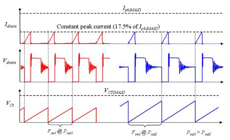
Figure 5. I<sub>drain</sub>, V<sub>drain</sub>, V<sub>Ct</sub>, at Different Output Loads in VCO Mode
