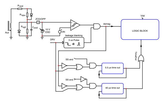
Figure 8. Zero-Crossing Detection Bloc Schematic
