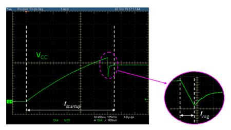
Figure 11. V<sub>CC</sub> Waveform During Startup
