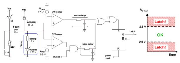
Figure 12. OTP/OVP Combination in NCP1380 A and B Versions
