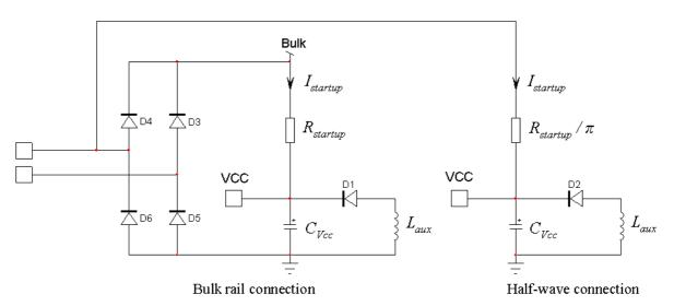
Figure 10. The Startup Resistor can be Connected to the Bulk Rail or to the Half Wave
